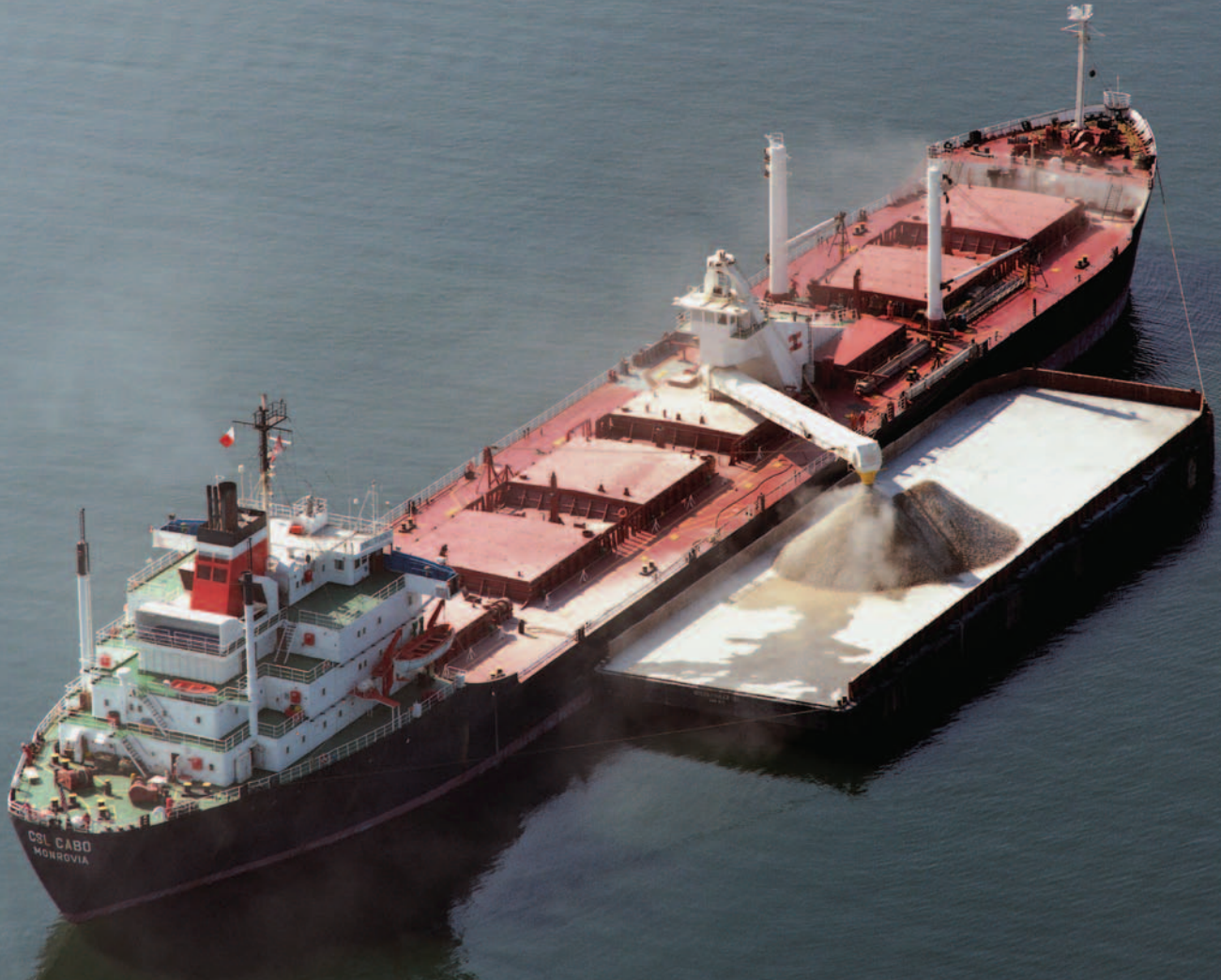
The CSL Cabo unloads gypsum into a barge alongside.
